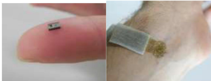
Figure 6: Wearable blood flow sensors based on the Doppler Effect
