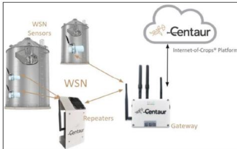
Figure 1: On-site system architecture diagram.
