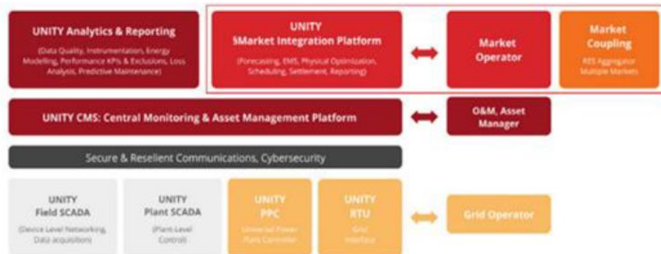
Figure 1: Schematic diagram of the Inaccess integrated VPP platform [8]
