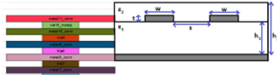
Figure 2: Microstrip line cross section
