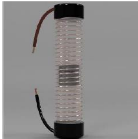
Figure 2. Rendering of an experimental electromagnetic microgenerator
