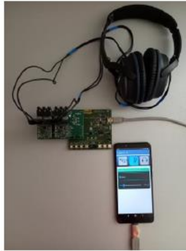
Figure 4: Setup implementation of the Adaptive ANC method
