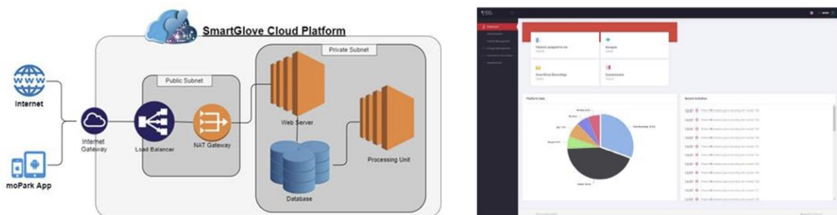
Figure 1. (a) SmartGlove Cloud Architecture, and (b) Main Dashboard.
