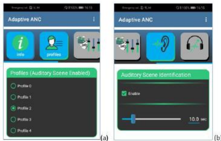
Figure 3: Android App GUI; Manual ANC profile selection (a), Automated Auditory Scene Identification algorithm enable and profile switch time setup (b)
