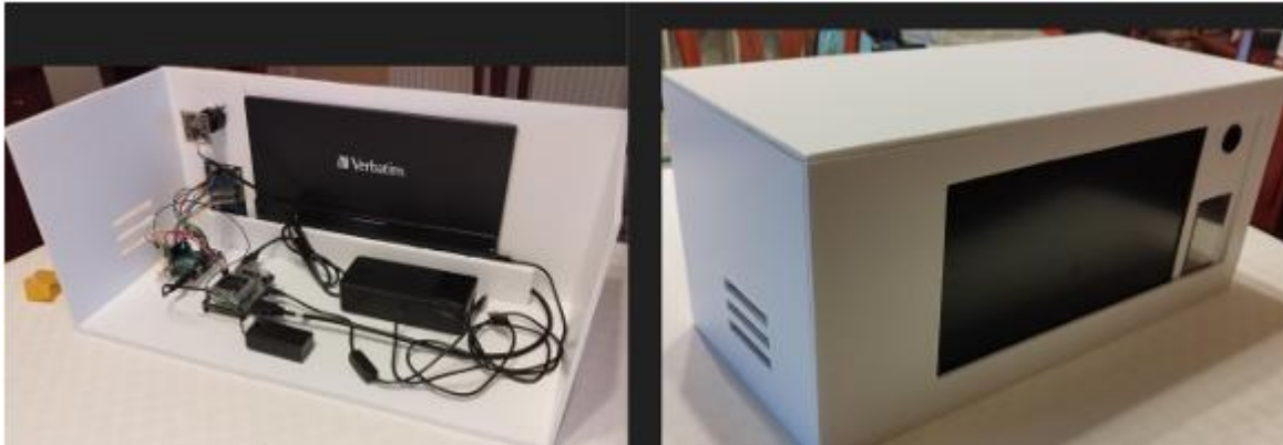
Figure 2: Back and Front panel of the Integrated device using the Coral TPU board, LCD screen and the display
